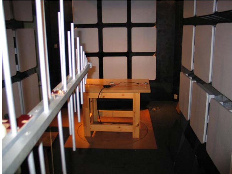
Photo 3. Set-up RF Radiated Immunity
